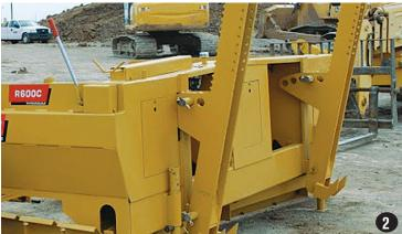
Hitch must be installed on the back of the spreader prior to attaching to dozer blade or bucket. Install bottom end first using the 1-1/2" pins following with the top one in the middle hole. Do same to other side and then put cotter keys in bottom pins.
