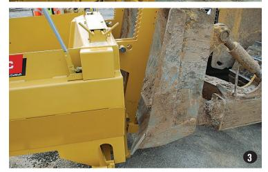
Position tractor at rear of spreader and place cutting edge of blade /bucket into spurs, located on bottom of the mounting brackets. Remove the two top pins from the mounting brackets to allow brackets to rest against the top edge of blade/bucket
