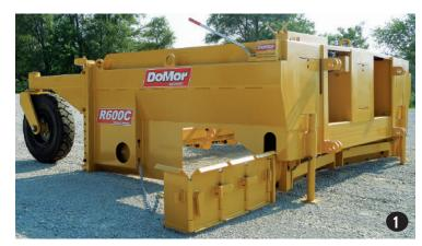
Spreader should be parallel with the ground and standing on the parking stands located at the back of the spreader. Wheels should be in the straight forward position.
