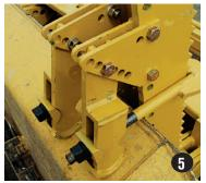
Place plate mounting clamp on top of blade/bucket back to determine position. Attach mounting clamp brackets. Slip clamp up into brackets; put "J" bolt through clamp and hook on front of spreader mounting brackets and tighten. Insert upper pins into nearest holes. After this has been done on both sides, lift spreader with tractor blade/bucket several times and the retighten.
